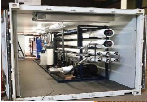
Gambar 1. Sea Water Reverse Osmosis (SWRO) berkapasitas 20.000 L/Jam.
